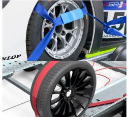
O Tie-down wheel straps Various types of tie-down straps are available to suit different loading applications, including wheel circumference straps that hold the vehicle safely and securely without straining suspension geometry. Easy to fit, with multiple built-in tie-down points.
