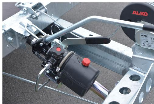
**O Hydraulic tilt-bed** reduces loading angles and can assist in ease of operation.
